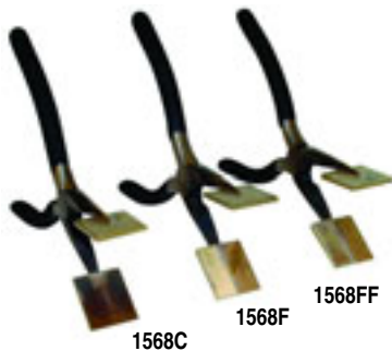
PATTERN IMPRESSING PLIERS Cat. No. 1568FF- Fish Fin/Bird Tail Cat. No. 1568F - Fine Leaf Cat. No. 1568C - Coarse Leaf Pattern plates mounted on top quality 8" (203mm) long-nose pliers for mashing molten rod ends. Leafmakers form a V-vein pattern on one side of the glass. A Fish Fin or Bird Tail impresser forms parallel grooves on both sides of the glass.
