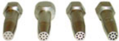
1560-HTM0 7 hole .031" 1560-HTM1 9 hole .040" 1560-HTM2 9 hole .049" 1560-HTM3 9 hole .055"
