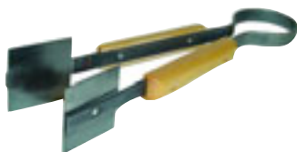
PARALLEL CLOSING GLASS FLATTENER Cat. No. 1579 - 9-1/2" (241mm) overall length, 2" (51mm) square x 1/16" (1.6mm) thick stainless steel pads mounted on a spring-loaded steel frame. Designed for parallel closing which maintains uniform thickness. Insulated with wooden handles.
