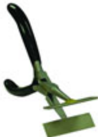
STAR MASHER Cat. No. 156905 Use to make a star murrini. Form a 3/4" (19mm) gather of glass, approx. 2" (5mm) long. Punty an end. Heat at pinch point and pinch along the cylinder side to form a star leg. Repeat as needed, then pull to desired diameter.
