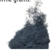
(-08) POWDER grains 0.2mm and finer
